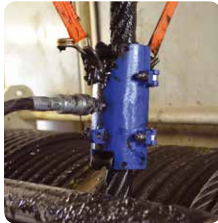
Newly installed wire rope lubricator on wire rope previously lubricated manually. Note: Even, clean penetrating distribution vs. uneven, messy coverage from previous method.
